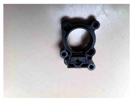
Remove the plastic "lock" insert
